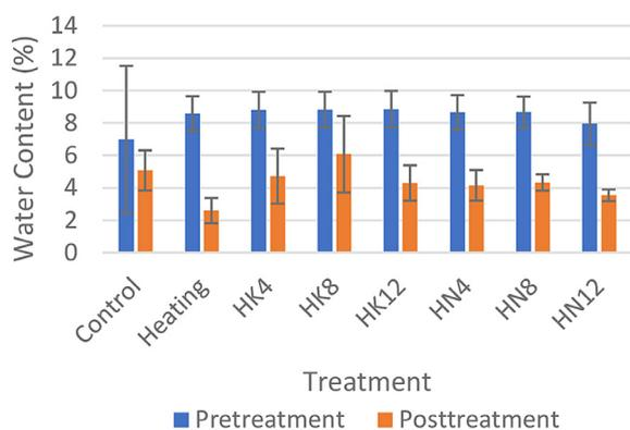
**Figure 2.** Water content of biochar activated by different treatments
