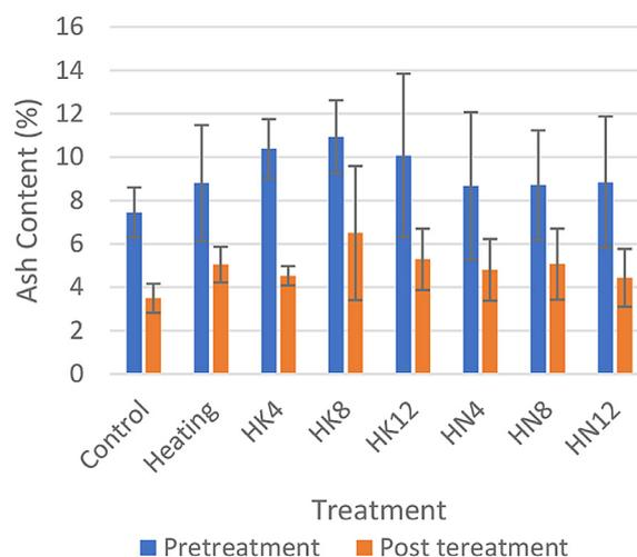
**Figure 3.** Ash content of biochar activated by different treatments
