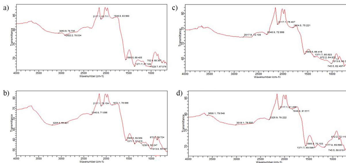
**Figure 8.** FTIR Biochar, a) Pyrolysis without activation; b) with NaOH post-treatment; c) with KOH post-treatment; d) with pretreatment
