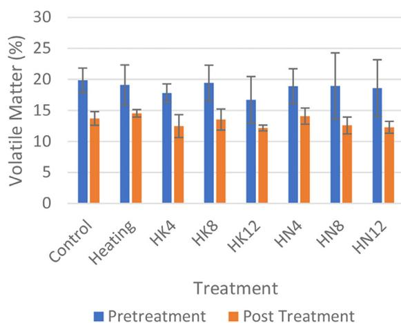
**Figure 4.** Volatile matter content of biochar activated by different treatments
