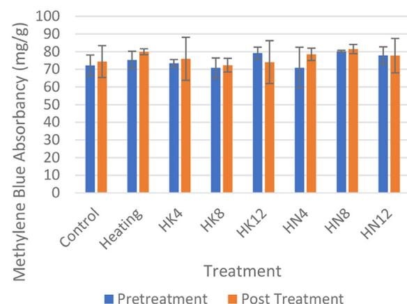
**Figure 7.** Methyl blue absorption of biochar activated by different treatments
