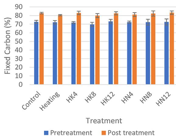
**Figure 5.** Carbon content of biochar activated by different treatments
