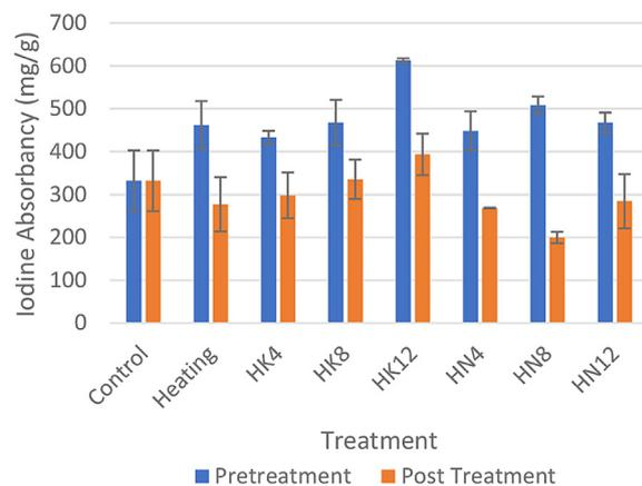
**Figure 6.** Iodine absorbency of biochar activated by different treatments
