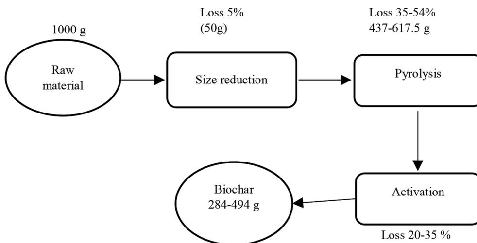
Figure 1. Mass balance of biochar production
